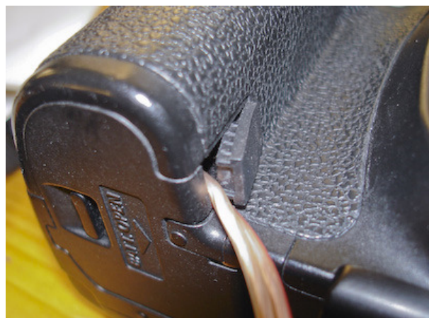
Left: The opened standard battery module showing the voltage converter (details found in the text below), Right: Cables feeding power to the camera using the empty battery body in the battery compartment of the camera which offers a cable opening for exter-
