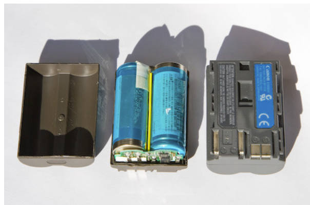
Left: open battery module with two lithium Ion cells, Right: The closed module shows the lengthy contact stripes on the left hand side of the battery case where the standard voltage of 7.4VDC is available
