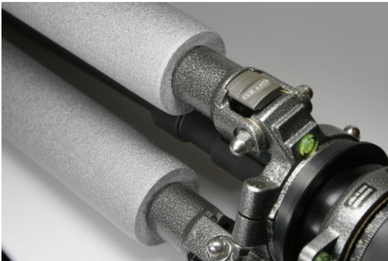
The upper leg segments are insulated with off the shelf insulation material used for water pipes
