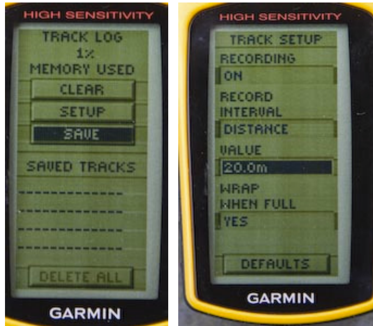
Left: Perceptual display of the log memory used for the track. Right: Setup of how to record the track; here it's set to record one track point every 20m
